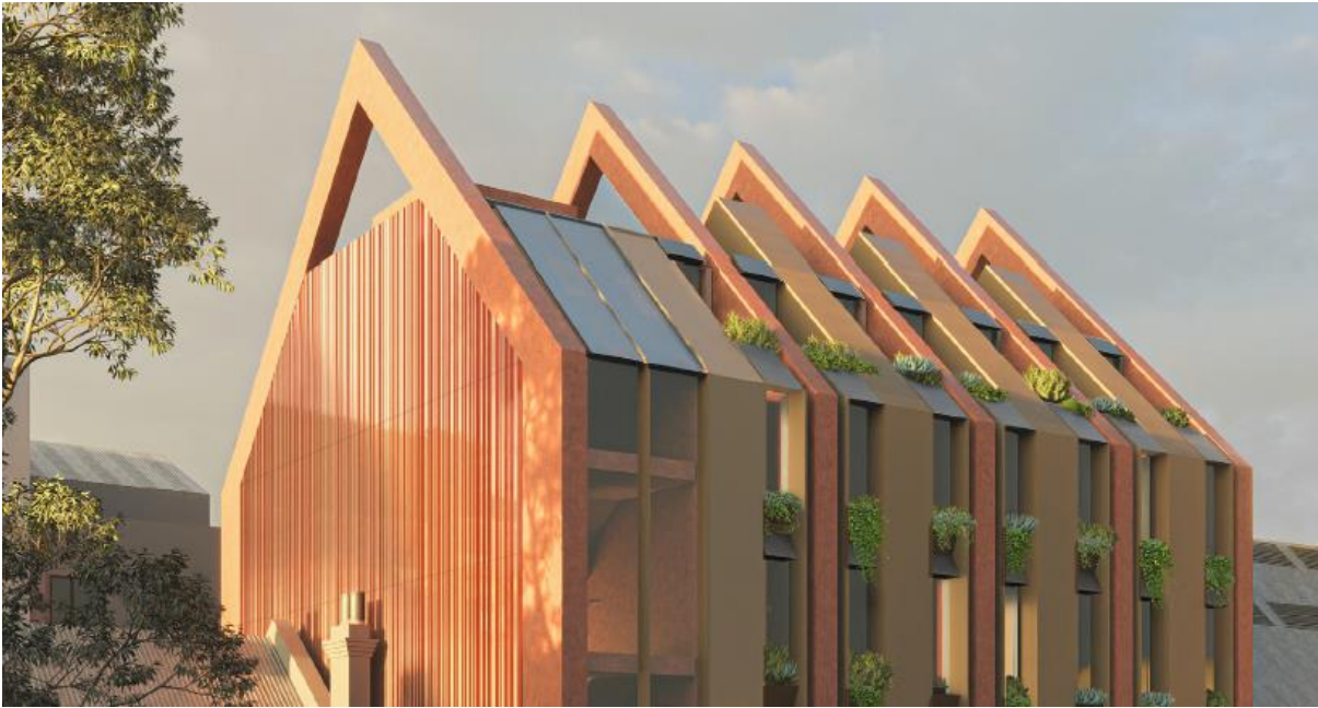
Figure 38: 3D perspective of west elevation illustrating columns and vertical exhausts integrated into the design and providing a greater solid to void ratio along this elevation to mitigate overlooking of residential properties to the west
